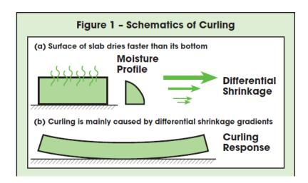
Thin slabs and long joint spacing will potentially increase the risk of curling and for this reason applications such as thin unbonded toppings need to have close joint spacings. This issue of close joint spacings can be undesirable in large industrial floor slabs because of, as previously mentioned, the increased risk of joint breakdown and increased maintenance.
